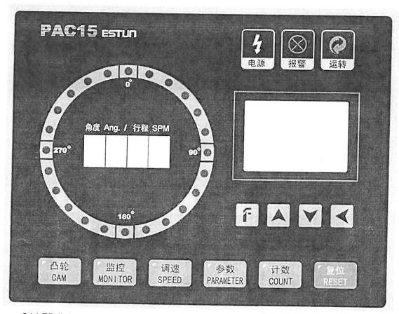
24 LED lights are used to indicate angle of crank. If the machine speed is over 150 SPM, the angle indicated by them does not reflect actual position.
