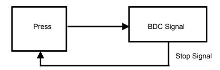
The device detects the BDC position normally in micrometers ( $\mu$  m), but it can be reconfigured to detect in units of 0.1  $\mu$  m in the initialization mode. This feature allows you to perform more minute detection even in press operations with less variation in BDC position.
