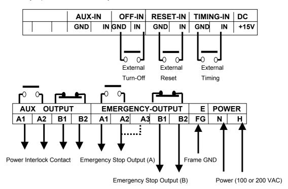
A3: As a power switch contact is provided between A1 and A3, the circuit between A1 and A3 is shorted when the power switch is turned off. Therefore, connecting a jumper between A2 and A3 makes it possible to start the press even with the device power turned off.
