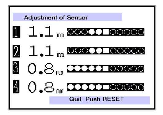
The bar display serves as a clearance gauge between sensor and approaching object.
