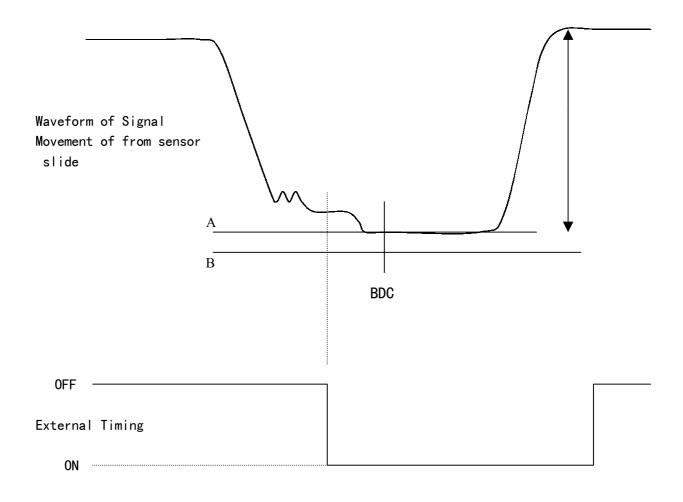
Normally the device detects BDC at the lowermost position (position B in the figure). By using the external timing input, it is also possible to detect BDC at a position where the timing signal is turned on (position A in the figure).
