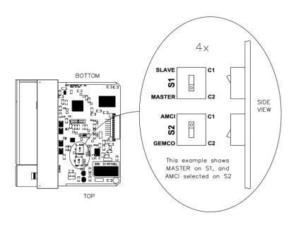
Step 1 (Master/Slave Selection) → Set dip switch (S1) to Master (On) position or Slave (Off) position.
