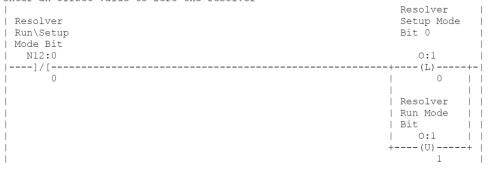
Rung 2:1 this rung sets the helm resolver into run mode when the panelview setup/run button is set to run mode; the helm resolver should be in this mode for normal operation
