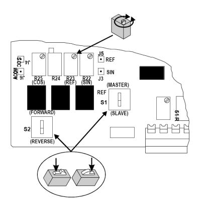
Step 1. Set dip switch (S1) to Master (On) position or Slave (Off) position.
