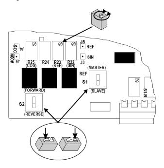
**NOTE:** For all measurements, use testpoint J6 for ground connection and make sure you are using a true rms meter.
