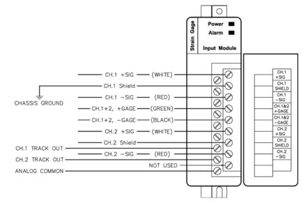
To ensure proper operation and high immunity to electrical noise, always use Helm strain gage cable.
