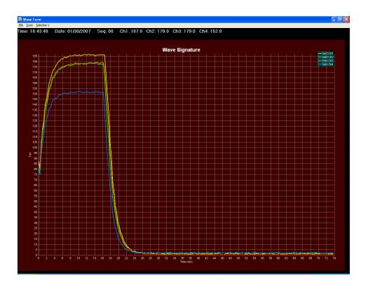
This screen allows you to view the waveform of the record, as well as the peak tonnages. From this screen you can zoom, and print the waveform.
