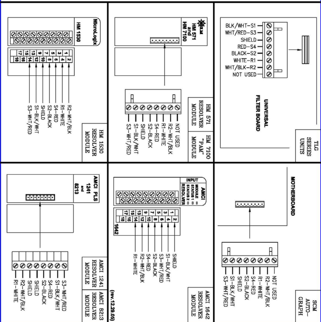
*HELM Model HR 1101-F, Resolver Cable Wiring*
