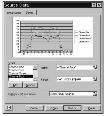
Then, select the contents of Column A. Once you have selected the values, click on the button below the X button in the floating window. You will now have an entry in the "Category (X) axis Labels" field, as shown below.
