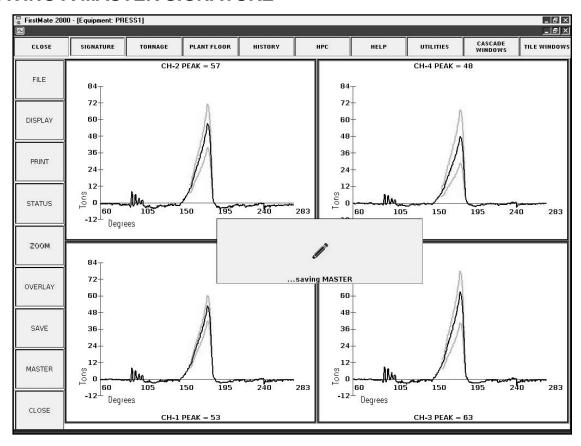
Pressing the MASTER button saves the current signature to a file named MASTER.WAV and this file can be displayed as an overlay on subsequent signatures. This feature allows you to compare each signature to a "good" signature and detect variations from the desired one. MASTER signatures can be displayed via the SIGNATURE ANALYSIS PANEL.
