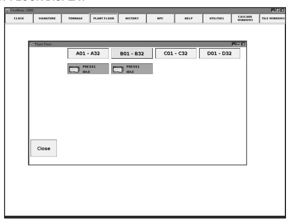
Plant Floor provides a view of all the instruments on the FirstMate network and allows you to quickly assess the status and current operation of each. It also provides a path to the Signature and Tonnage screens for any instrument you choose. Each instrument is displayed in the window.
