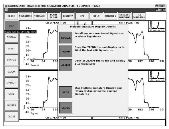
Selecting the FILE button opens the Multiple Signature Display Panel and allows you to access the File features of FirstMate 2000:
