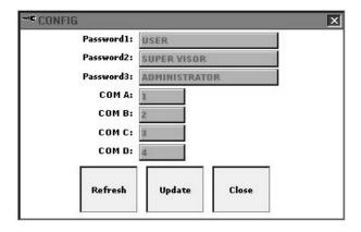
Firstmate 2000 has three levels of password protection controlling the access to its functionality:
