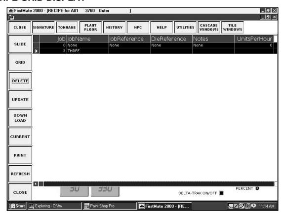
This is the stored recipe grid display showing all stored recipes in a spreadsheet display. Clicking on a recipe line opens the recipe editor and allows you to modify the selected job. Use the GRID button to toggle this feature ON/OFF.
