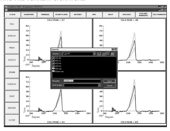
Pressing the SAVE button opens the Windows "Save as" panel. You can save the current signature to any location and name. Note that signature file extensions .WAV should be maintained.
