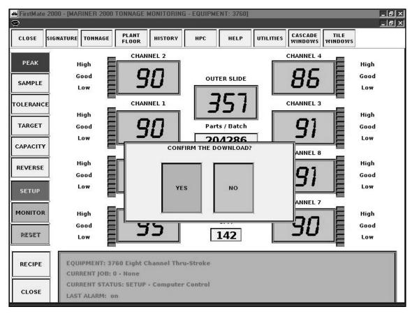
FirstMate 2000 displays the current instrument mode using active buttons on the left side of the window. For instruments that have the capability to accept downloaded mode changes you may send these changes by clicking on the SETUP or MONITOR button. This opens the CONFIRM PANEL and clicking on the YES button sends the download to the instrument. When the instrument is re-polled the mode change will be displayed. Only instruments with proper features will respond to this download.
