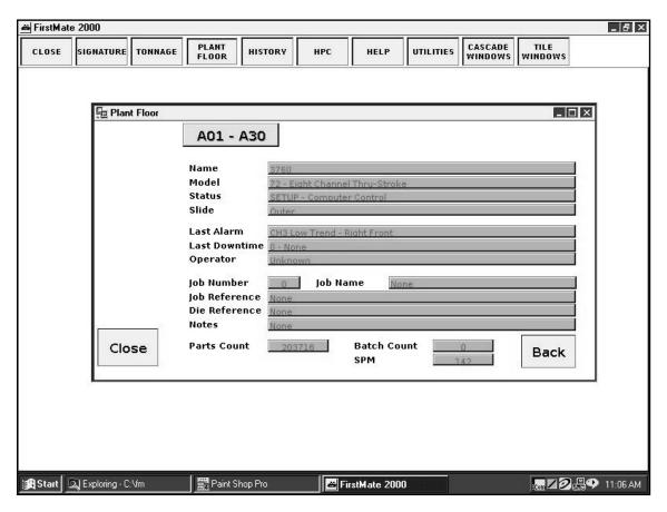
EXPLORE display current information for the selected instrument. Click CLOSE to return to the Plant Floor display or BACK to return to the menu bar. TONNAGE opens the Tonnage Display window - SIGNATURE opens the Signature Display window. RECIPE opens the Job Recipe display for this instrument.
