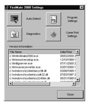
The command buttons located at the top of the dialog box perform actions such as setting up the communication ports, performing diagnostics, and autodetecting instruments that exist on the system.
