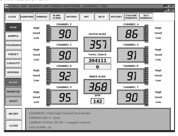
**Tonnage** is displayed on this screen which also contains related features. Each channel of tonnage is displayed in a separate box and the total tonnage is shown in the center. When the total channels exceed four, the display is divided into two sections representing four channel instruments with separate totals. Clicking the mouse on any channel of tonnage shifts focus to Signature Display.
