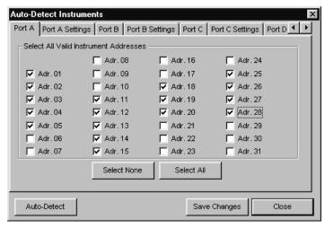
Example: From the Port A tab, select Addresses 1, 2, 3, 4, 5, 11, 12, 13, 14, 15, 18, 19, 20, 25, 26, 27, and 28. This will perform a scan looking for 17 instruments on Port A. Then set the port's settings. Click on the Port A Settings tab and enable the Communications Port then specify the Maximum Baud Rate to be 57600 bps.
