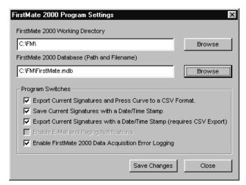
From the main FirstMate 2000 Control Panel, click on the Program Settings button. This will load the Program Settings dialog, and will allow you to change the file paths for FirstMate to use and select optional signature and data acquisition features.
