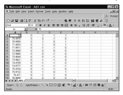
The file should have numbers in the first five columns. Column A is the Resolver Angle if it is a TSM Instrument; otherwise, it will display the window time in milliseconds. Column B is the Tonnage Values at the corresponding point in Column A. Therefore, the first value of Column B states that there was no tonnage at 70 degrees. Column C, D, and E are Channels 2, 3, and 4 respectively. There will be 448 points sampled for each channel of the signature.
