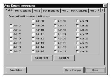
The tabs, at the top, allow you to specify the settings for the four communications ports to be used by FirstMate 2000. The "Port X" tabs (where X is either A,B,C, or D) allows you to specify which instruments are present at that address for that serial communication line.
