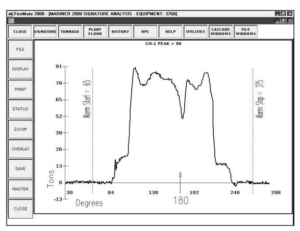
Any Channel Display may be resized to a full window by clicking on the signature display. This feature allows you to focus on one channel and provides a more detailed view of the signature. Click on the display a second time to return to the signature's original size.
