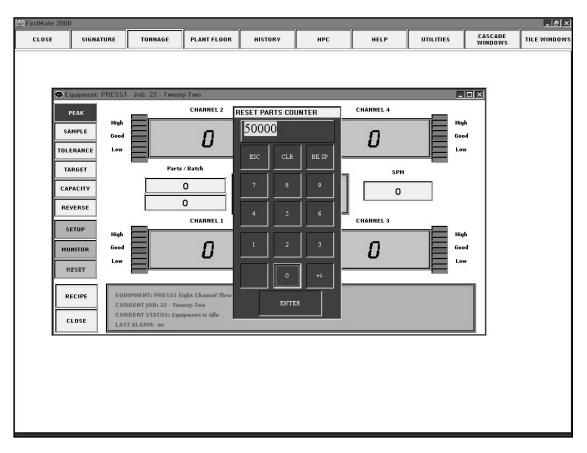
The Parts and Batch Counters can be set from the Tonnage Display. Click on the counter display to open the numeric keypad. Enter the values on the keypad and then press ENTER to confirm the download. ESC closes the keypad without saving an entry. Use CLR to clear the display and BKSP to backspace and remove the character left of the cursor.
