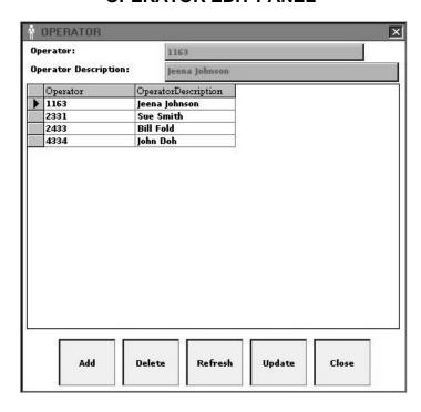
This is a simple table containing two fields: Operator and Operator Description. The Operator field corresponds to the Badge ID on HPC units and is the Operator Name on Autographs. This table provides an identifier to supplement the Operator Name. Enter the information in the green boxes and click on the desired editing function. You can position the cursor on any row in the table prior to editing.
