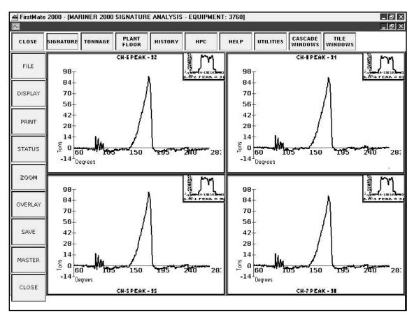
SWITCH INNER/OUTER reverses the signature sizes in the channel display windows. The larger sized display is drawn in the smaller window and the smaller display is drawn in the larger window. Clicking the button a second time returns all signatures to the original sizes. This feature works best with double action presses with outer and inner slides.
