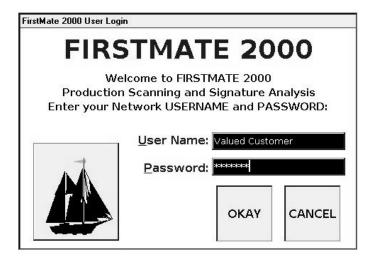
The startup screen for FirstMate 2000 requests a USERNAME and PASSWORD. Three levels of passwords are available controlling the level of usage within FirstMate. Entering a user name and password may be omitted if no security is desired.
