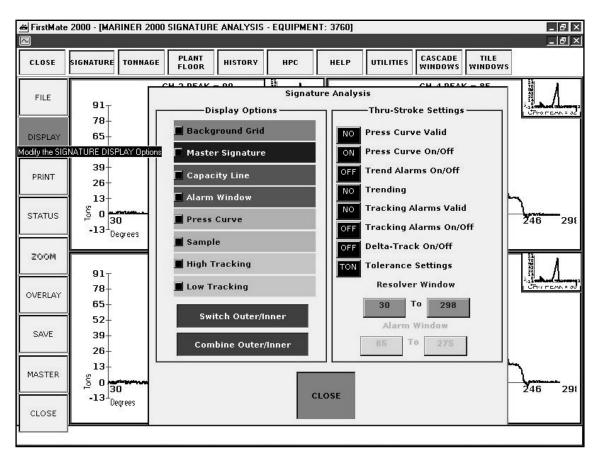
The SIGNATURE ANALYSIS PANEL provides the platform for controlling the display features of FirstMate's Graph Windows. These features are divided into three types: Standard, Thru-Stroke and Eight-Channel. Standard features are available for all types of equipment; Thru-Stroke is only available when the current instrument is a TSM unit. Eight-Channel features are available for equipment having more than four channels – typically double action presses.
