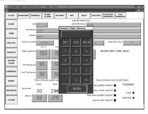
Clicking on any field opens a keypad and allows you to change the values for this instrument. Text fields have a full keypad and numeric ones are limited to digits. The switch settings can be changed directly. Once you have edited these values you can launch the download with the DOWNLOAD button.
