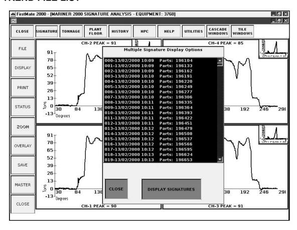
The Trend File List Box displays the records in the TREND and ALARM files. These files contain the last four hundred, standard and alarm signatures respectively. They are arranged by date, time and part number. Use the slider at the right to move up or down through the list. Select one to ten signatures by clicking on the desired listing. When you are finished selecting signatures, click on DISPLAY SIGNATURES to start graphing your selections.
