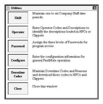
This panel has five buttons that provide access to Utility Table Maintenance functions. These functions edit the utility tables in the Access Database, FIRSTMATE.MDB.
