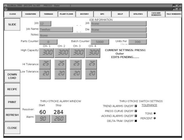
This is the Job Recipe display. It can be opened from the Menu Bar in Plant Floor of from the Tonnage display. This is where you enter information to download to an instrument. This is also the place where you set up the Job Recipe Database containing your Job files. The display shows the current settings for the instrument.
