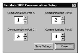
This dialog assigns serial communication port to FirstMate 2000 Ports. You can setup a port to use COMM 1 through COMM 9 (assuming you can assign nine ports without any conflicts with other hardware in your system.) It is possible to link two FirstMate ports to the same communication port, as long as there are no repeats in EIC addresses on that port. If you are going to use less then four ports, you can assign the unused ports to any
