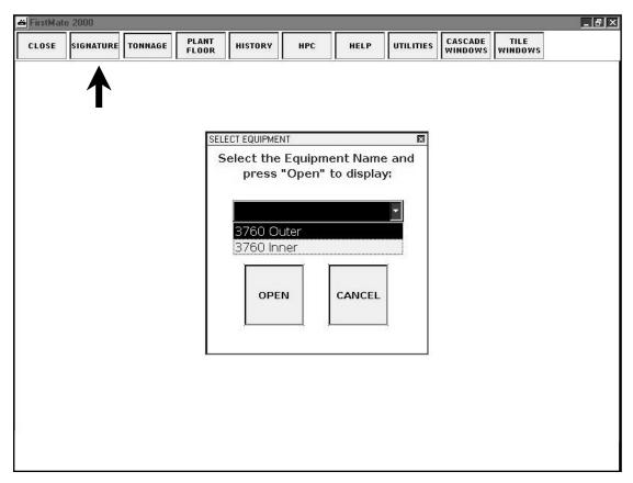
Clicking on the SIGNATURE button on the Main Menu opens the SELECTION PANEL that allows you to choose an instrument for Signature Analysis. Use the dropdown list box to select the equipment name and then click OPEN to display this instrument's Signature Analysis window. CANCEL closes the Selection Panel without opening a display.
