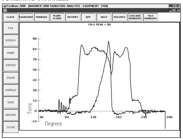
Channels 1 and 5, 2 and 6, 3 and 7, and 4 and 8 can be combined using the COMBINE INNER/OUTER button. This feature is useful when displaying signatures from double action presses where the inner and outer slides have related forming forces. The combined channels are graphed together. Clicking the button a second time returns the signature display to its original settings.
