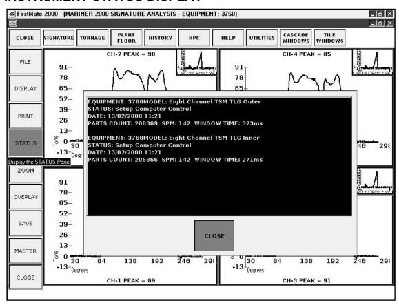
STATUS opens a display panel providing current information for the instrument displayed in this Signature Display window. Information on this display is updated as the instrument is polled. For instruments with five or more channels, the status is displayed separately for Channels 1-4 and 5-8. Click on the CLOSE button to hide the Status Display.
