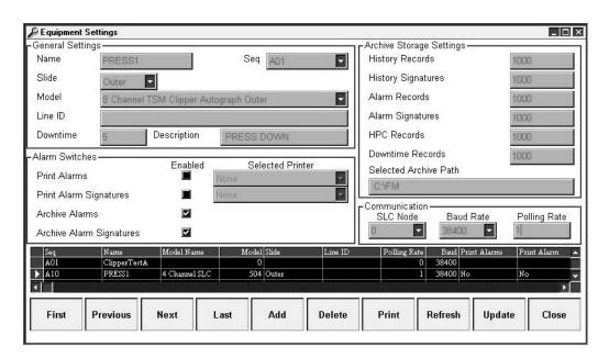
Use this screen to modify the EQUIP table controlling all features for each piece of equipment polled by FirstMate 2000. Use the **First**, **Previous**, **Next** and **Last** keys, or the grid slider bars to move through the table. Use the **Add**, **Delete** and **Update** keys to modify the table, clearing edits with the **Refresh** key if necessary. Generate an equipment list with the **Print** key.
