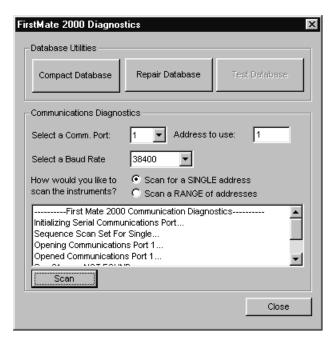
The Diagnostics dialog provides a simple mechanism for testing serial communications lines for the presence of a specific instrument. This allows you to check the integrity of the communication cable and/or the proper operation of the instrument's EIC card.
