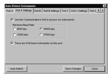
There are four tabs labeled "Port X Settings" (where X is either A,B,C, or D.) These tabs allows you to configure which ports you would like to use with FirstMate and assign the maximum baud rate to be used on each port.
