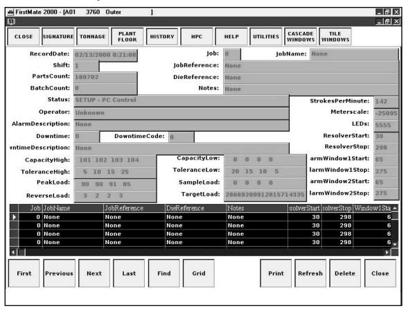
This is the History Database Display for the selected instrument. All history records are shown in the grid at the bottom of the window and the current or selected record is shown in the display's fields. Control buttons are available along the bottom of the display. This history is a snapshot of the database when the window is opened. It does not update unless you refresh the display.
