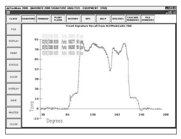
Selected Trend Signatures are graphed in overlay fashion using a different color for each signature. The Date, Time, Parts Count, and Peak Tonnage values are listed in matching colors at the side of the Signature. Tonnage is scaled to the highest peak value for all selected signatures. Degree or Millisecond Look Windows are scaled to the first signature in the selected list. Selecting signatures with large differences in peak value or look windows can result in unreadable displays.
