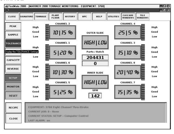
This picture shows the **Tolerance Alarm** settings. The values are **HIGH LOW** for each corner and represent **Percent** (%) in this example. Parts Count and Batch Count are displayed in the center of this window. Strokes per Minute is shown at the bottom. The green panel displays current Status information: Equipment Name and Model, Current Job Name and Number, Current Status of the instrument, Last Alarm condition, and Last Downtime.
