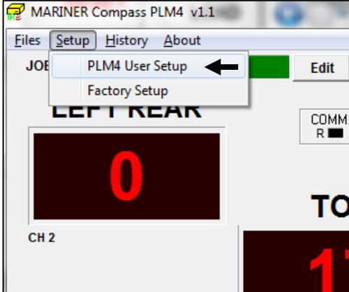
When you connect new load cells to the Compass PLM4, you need to set up the Compass PLM4 with proper parameters for each load cell connected in PLM4 User Setup screen.
