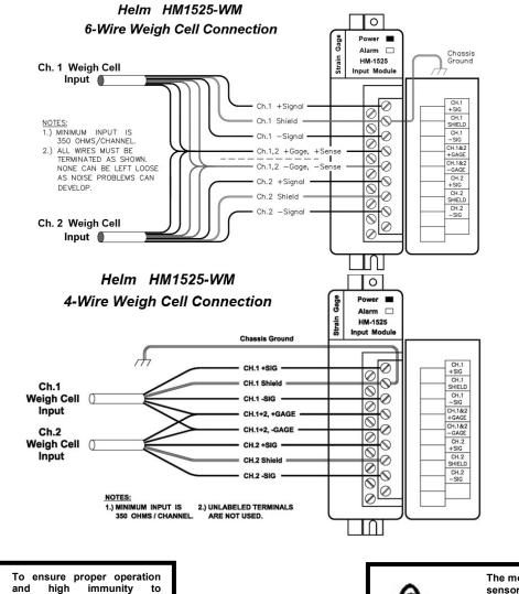
The module can support up to two sensor inputs.
