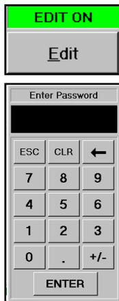
Before you are able to make any changes on the settings in this screen, you have to enable Edit mode first. To do so, click on Edit button and enter a password to enable the Edit mode. Depending on the password clearance level, restrictions will apply.
