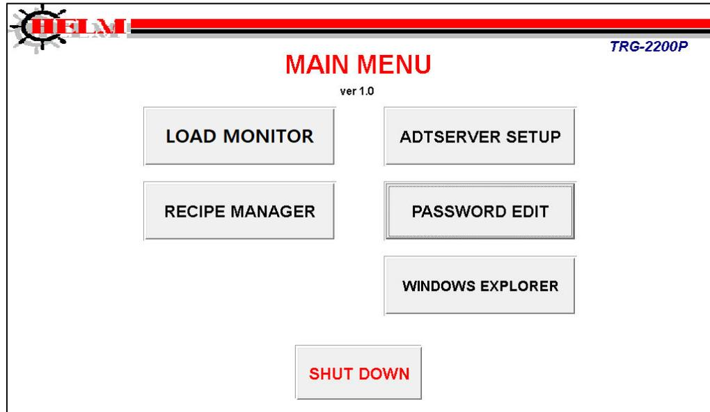
**LOAD MONITOR** – This is the main load monitor screen where you can view the peak loads, load signatures, change Alarms settings, etc.
