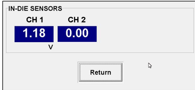
This screen is to help calibrating a PTM-1 module to get a proper reading from the load sensors connected. Each number is the voltage from PTM-1 track out signals for each channel. It displays sensor balance voltage if PTM module's function switch is in OFF position and Cal voltage if the switch is in CAL position.
