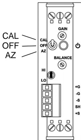
1. Move the 3 position switch of the PTM module to Off position
