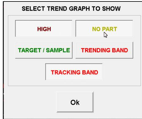
You can add/remove different types of trend graphs to overlay on the signature screen. When the button is pushed in, the option for the graph is added. Click again to remove it.
