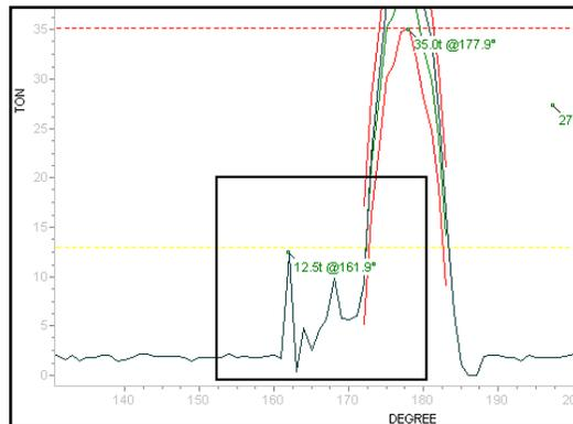
To select an area to zoom in: Press touch screen (and keep pressed) at top left area of desired part of wave to zoom in, and drag finger at a diagonal down and to the right. A box will be drawn and finger followed as the touch screen is pressed. Release touch screen to draw zoomed-in part of the wave.
