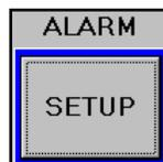
Click on ALARM SETUP button to bring up CURRENT ALARM SETTING screen where you can set or change the current alarm settings and download the new settings to the system to take effect. You can also stores any change you made in this screen to Recipe database easily. Refer to CURRENT ALARM SETTING for details.
