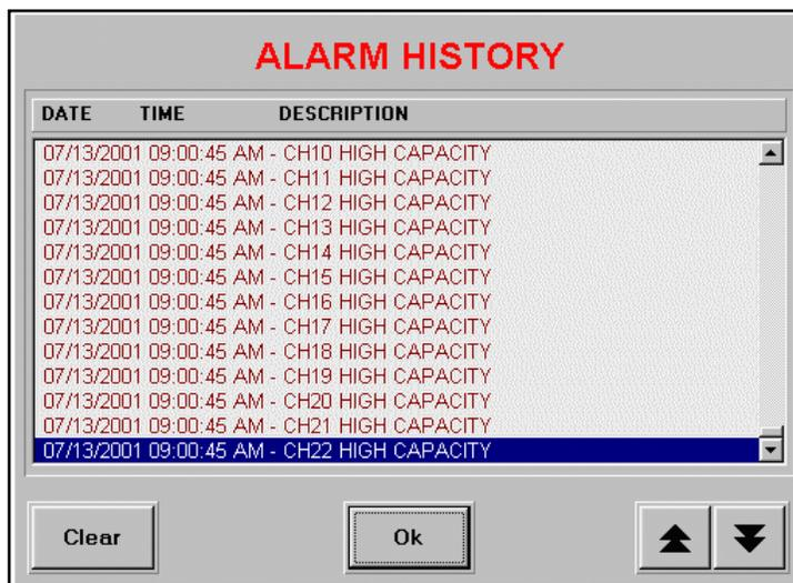
You can view up to last 1000 alarm messages recorded with date and time stamp each. Use the scroll bar on the right side of the list box or arrow buttons on the bottom to scroll up and down the list. Use *Clear* button to empty all messages.
